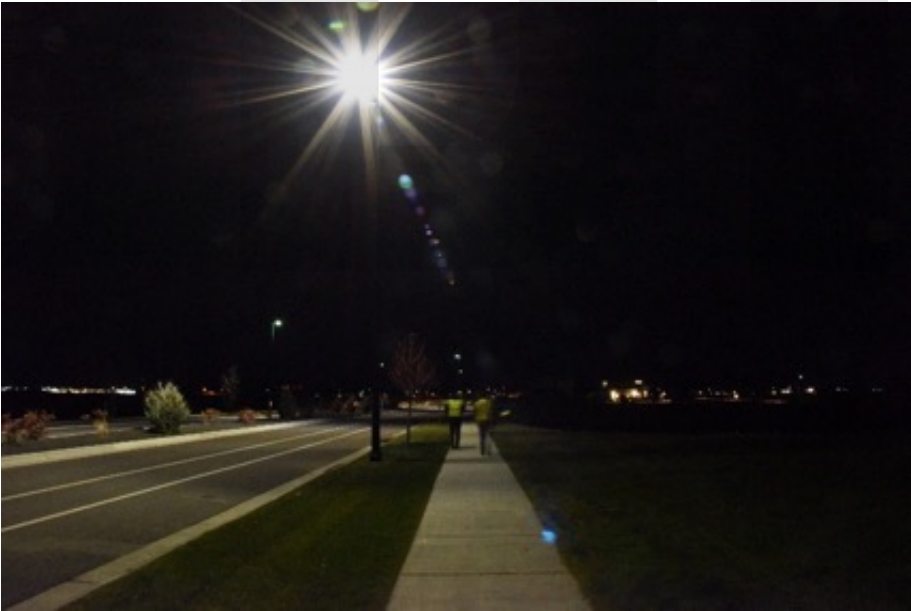
This lighting option has significant glare and prioritizes the vehicle right of way, creating visibility and perceived safety issues. (Source: SLC Street Lighting Masterplan)
