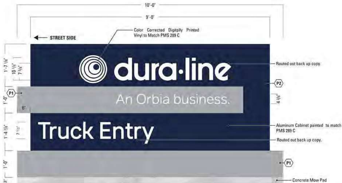
1 SIGN 05 - D/F INTERIOR ILLUMINATED MONUMENT SCALE: 3/4" = 1'-0" [1:16]
