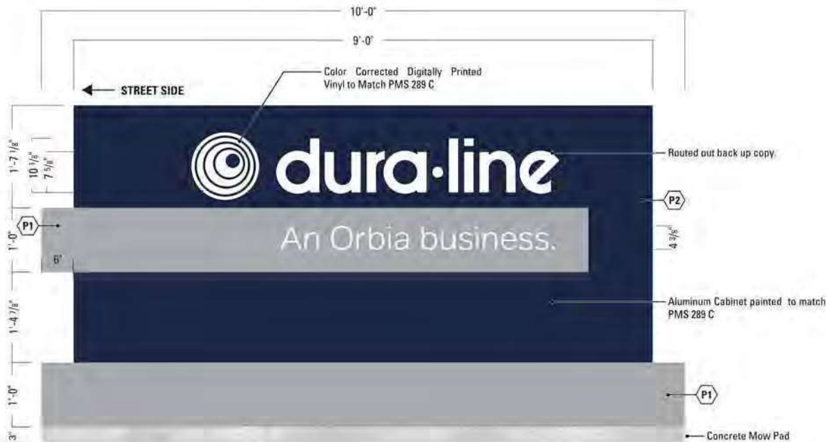
1 SIGN 04 - D/F INTERIOR ILLUMINATED MONUMENT SCALE: 3/4" = 1'-0" [1:16]
