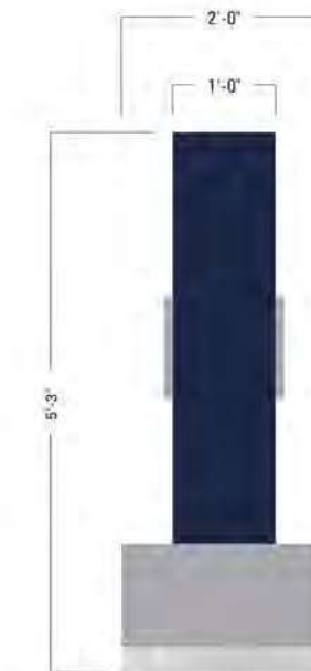
2 SIGN 04 - SIDE VIEW SCALE: 3/4" = 1'-0" [1:16]
