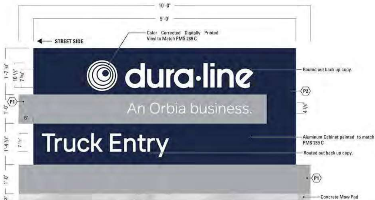
1 SIGN 05 - D/F INTERIOR ILLUMINATED MONUMENT SCALE: 3/4" = 1'-0" [1:16]
