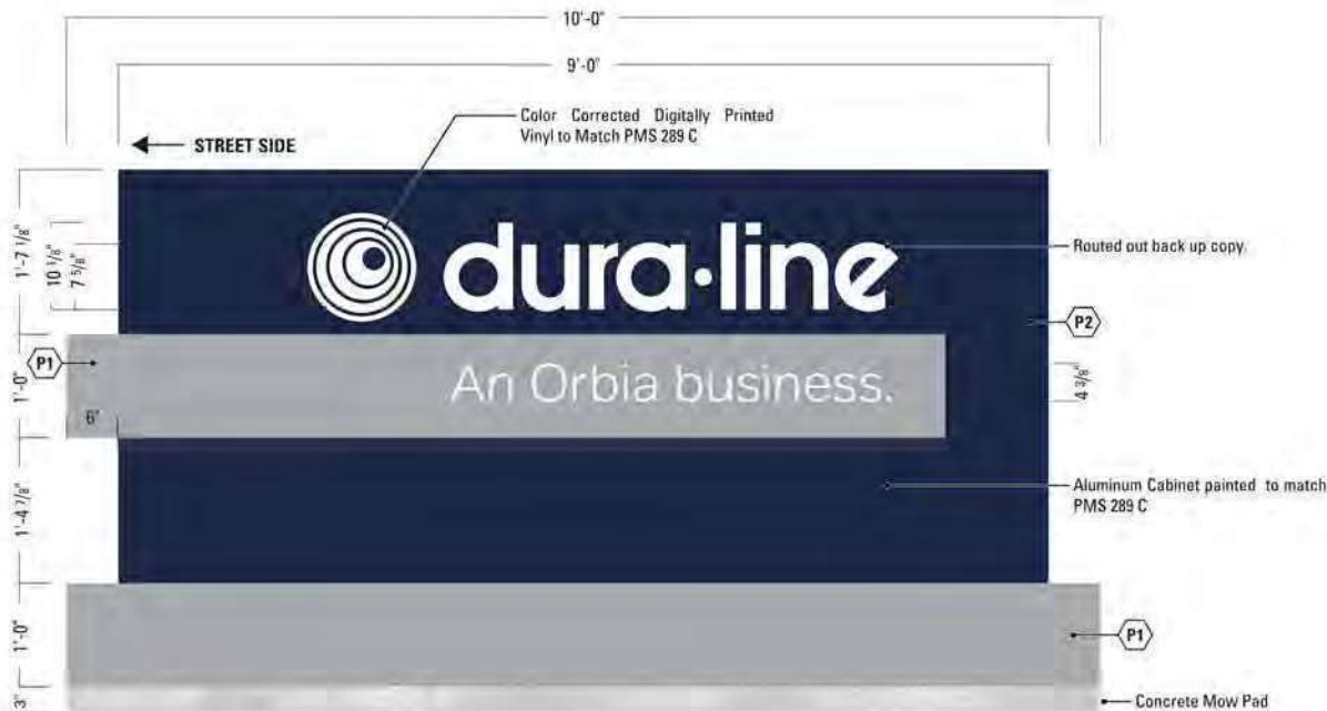
1 SIGN 04 - D/F INTERIOR ILLUMINATED MONUMENT SCALE: 3/4" = 1'-0" [1:16]
